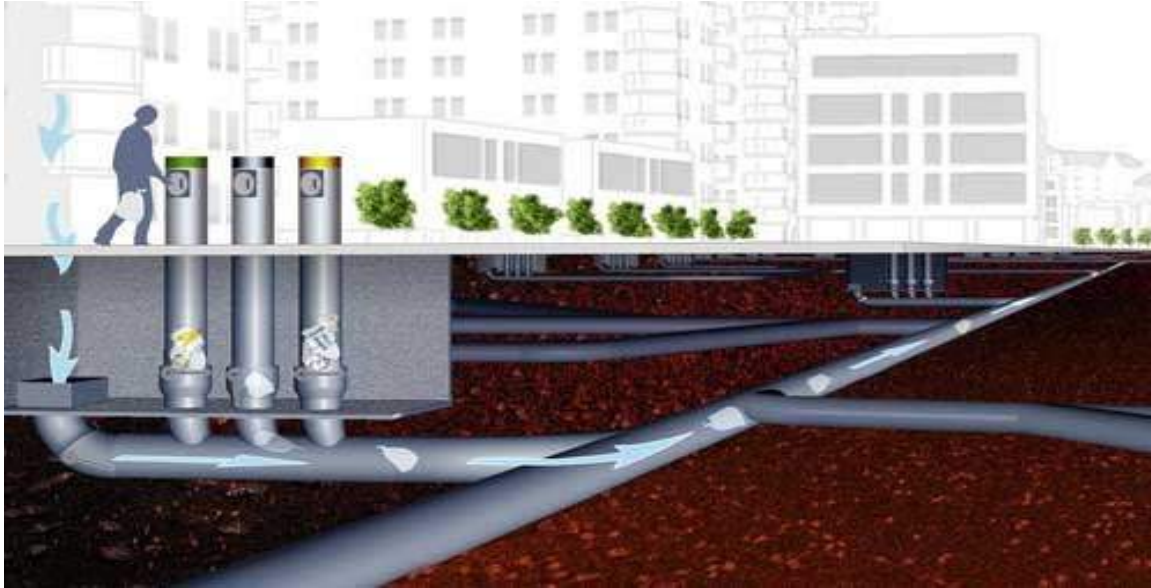
Figure 18. Vacuum Waste Collection Systems eliminate need for waste hauling trucks driving across site daily, and support higher waste diversion rates, and opportunities for additional graywater supply from organics. Communities such as Hudson Yards and Roosevelt Island both in New York are using these systems. http://motherboard.vice.com/read/should-new-york-city-expand-its-network-of-trash-sucking-vacuum-tubes ; http://www.greenerideal.com/lifestyle/0213-automated-waste-collection-sucks-but-thats-good/
